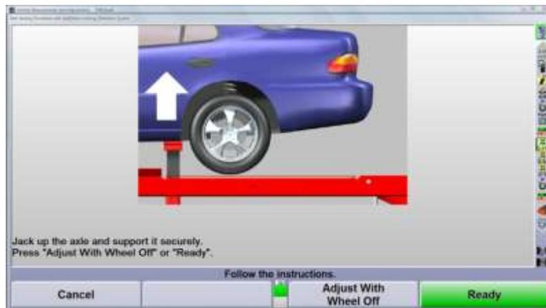
Adjust the camber or caster angle as needed.
