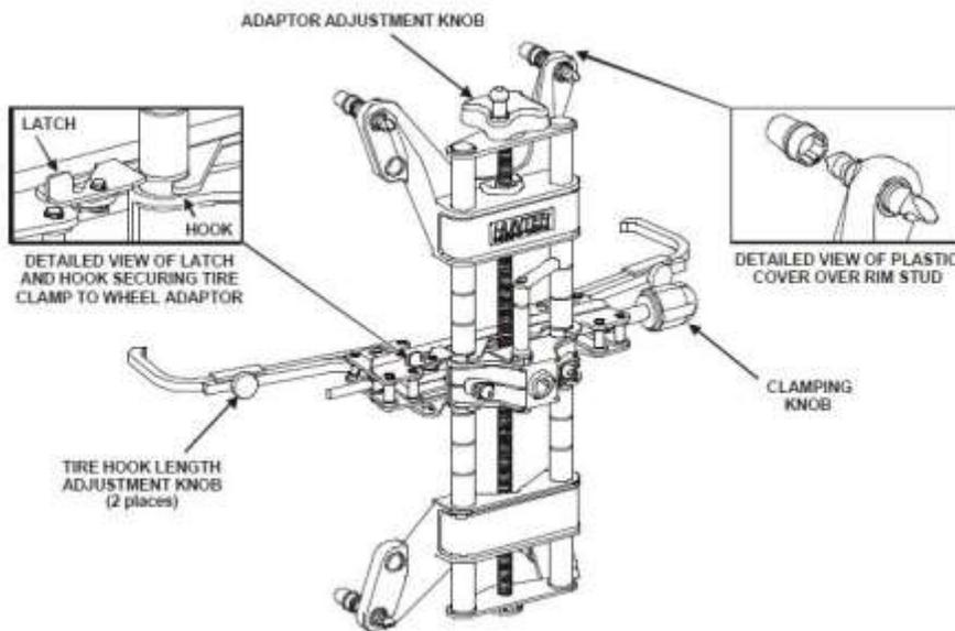
Install plastic covers over each rim stud to protect the face of the wheel.
