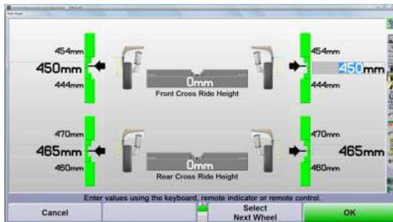
If the ride height was corrected, enter the measurements again. Press K4 "OK" to continue
