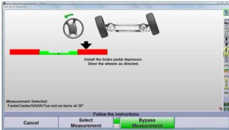
Steer to the left as directed until the arrow is in the lower valley of the graph. Hold the wheels still until the bar graph changes.
