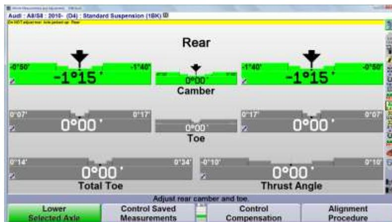
Press K1 "Lower Selected Axle" when adjustment is finished.
