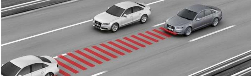
The Adaptive Cruise Control system is a radar-aided proximity control system, with stop & go ability. Two radar sensors are now located in the front end of the vehicle looking ahead.
