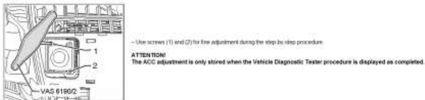
**The ACC adjustment is only stored when the Diagnostic tester procedure is displayed as complete.**
