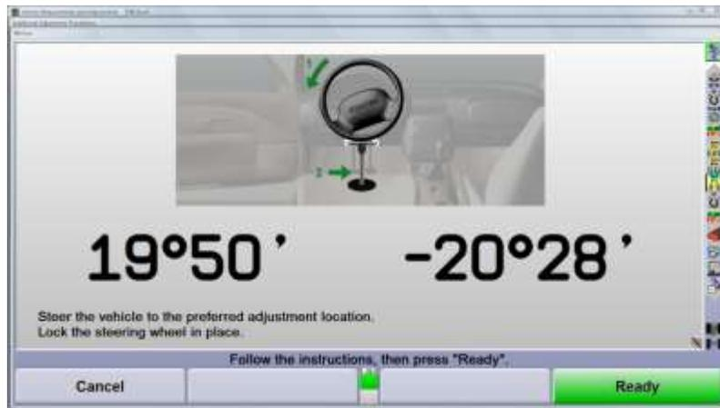
Press K4 "Ready" when the front wheels are secure.
