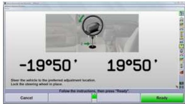
Once selected, the front wheels may be steered and locked in the steered position to access the adjuster. This saves time and aggravation when the toe adjuster is in the upper wheel well.
