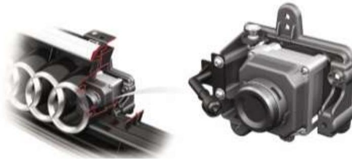
The remote infrared technology looks ahead up to 984 ft, depending on the driven speed. Because the system reacts to the heat emitted by objects, people and animals are generally displayed conspicuously bright, while the cool road remains dark.
