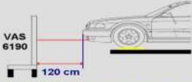
Assemble the VAS 6190, VAS 6041 with VAS 6041/1 or VAS 6430 calibration fixture and set it approximately 120cm (+/- 5cm) in front of the vehicle.
