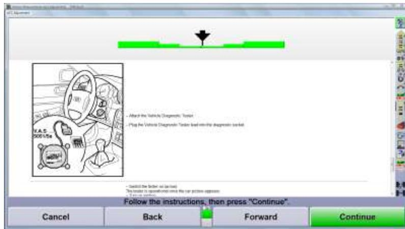
Follow the aligner's screen instructions, which guide you through diagnostic tester screens. Physical adjustment of the radar system is made by adjusting the mounting plate screws.
