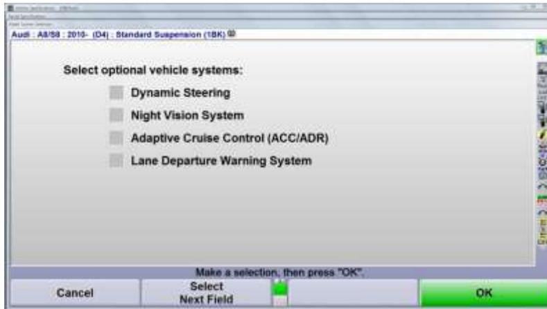
Place an "X" in the appropriate vehicle systems for the vehicle being aligned.
