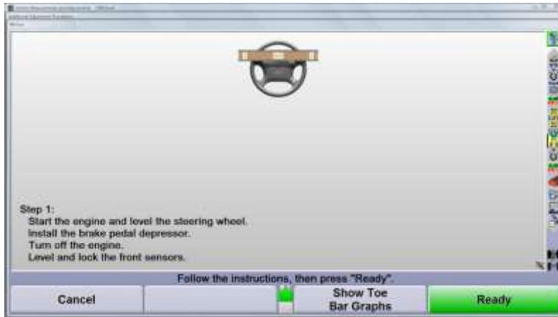
Enter WinToe® from the "Make Additional Adjustment" softkey or through the context sensitive drop-menu obtained by clicking on the steering wheel icon on the front toe bar graphs.
