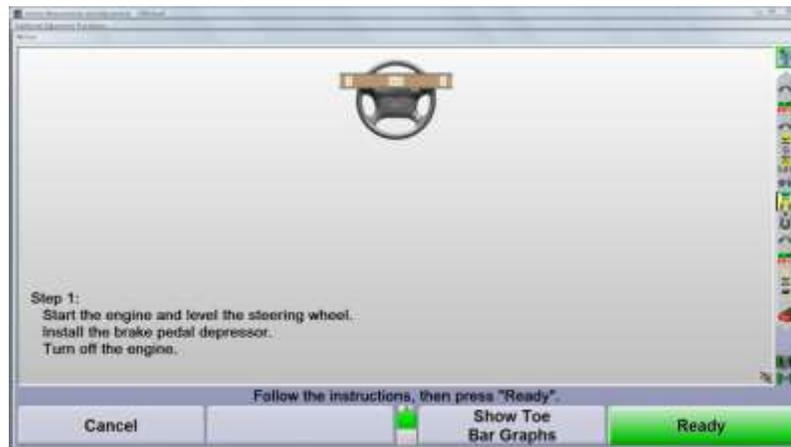
Follow the screen instructions to adjust toe without using a steering wheel holder.
