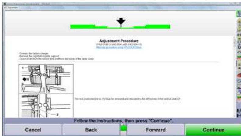
Connect the battery charger, remove the access cover and clean all dirt off the sensor lens and inside of radar cover.
