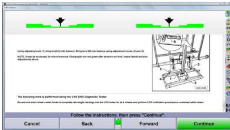
Record and enter wheel center fender to turnplate ride height for all 4 wheels. Perform LDW calibration procedures contained in the tester.
