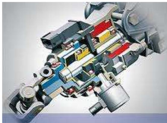
The dynamic steering and electronic stability systems work in tandem to provide a safe and stable driving experience. If electronic sensors determine that you're going too wide into a sharp turn, they will tighten up the steering ratio to put the vehicle back on course with a smaller movement of the wheel.
