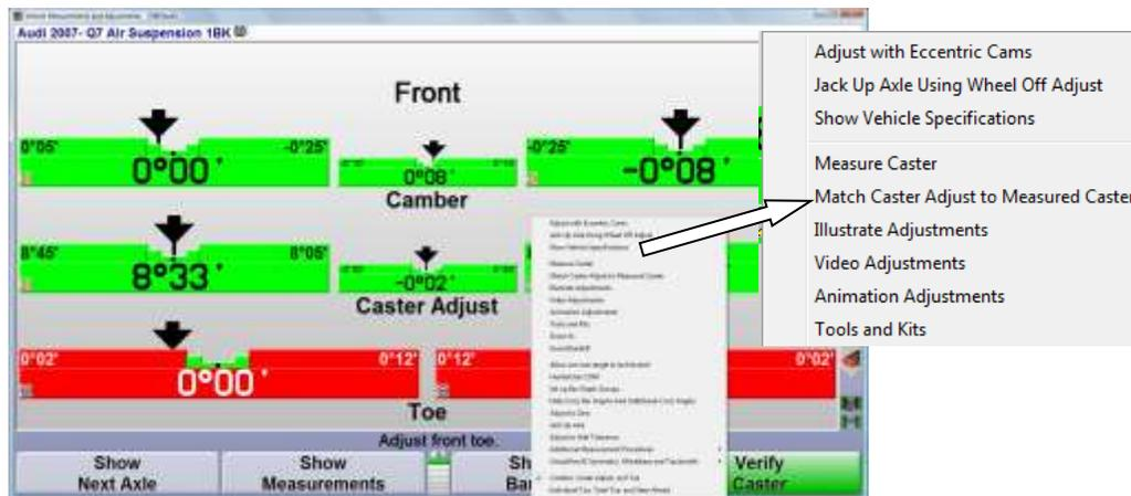
Conventional sensors: Adjust the level condition of the front sensor until the last measured caster value is displayed. Lock sensor securely.
