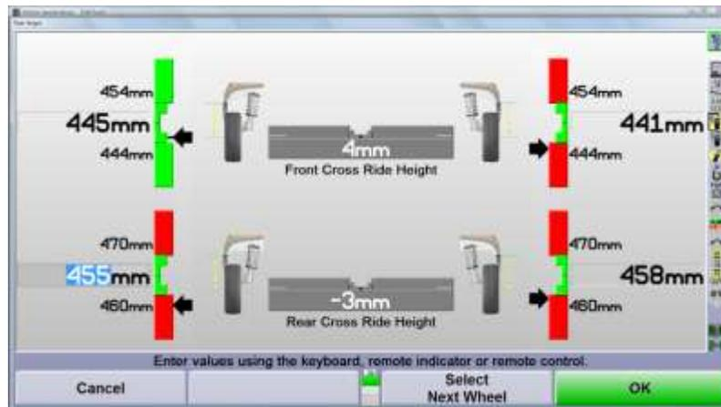
If the ride height is not within specifications, consult the repair manual for proper use of the Vehicle Diagnostic Tester. Correct the ride height using the Vehicle Diagnostic Tester.
