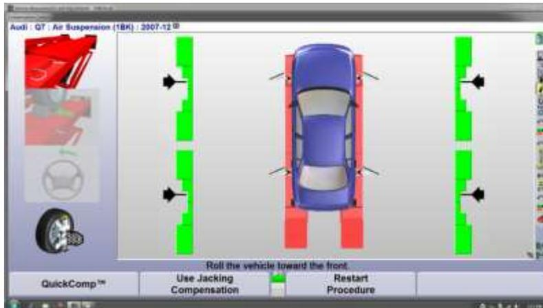
Roll the vehicle using the left rear tire until the bar graphs are green and the arrows are well within the green area of the bar graph. Hold the vehicle until the bar graphs change.
