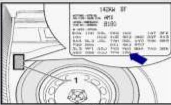
Various suspension versions are available as optional equipment. These are identified by factory codes listed on the vehicle data label.
