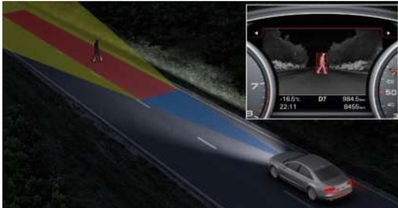
Audi's night vision assistant uses a thermal imaging camera sitting behind the four rings at the front of the car. A computer transforms the information from the camera into images and displays them on the display located between the instruments.
