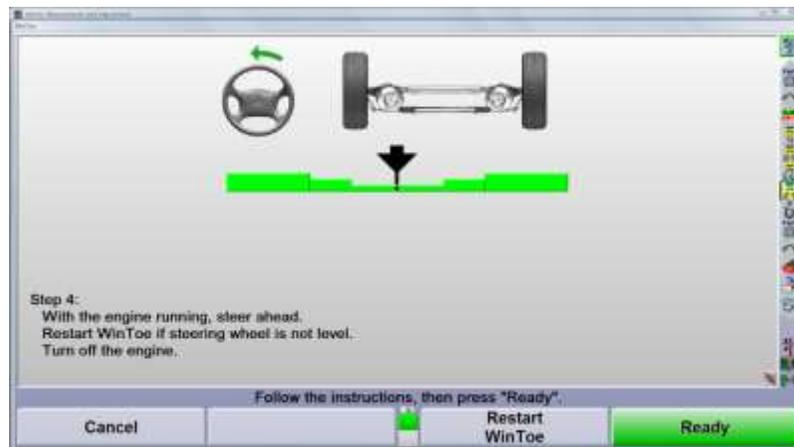
If the steering wheel position is acceptable, press K4 "Ready." If the steering wheel position is unacceptable, press K3 "Restart WinToe".
