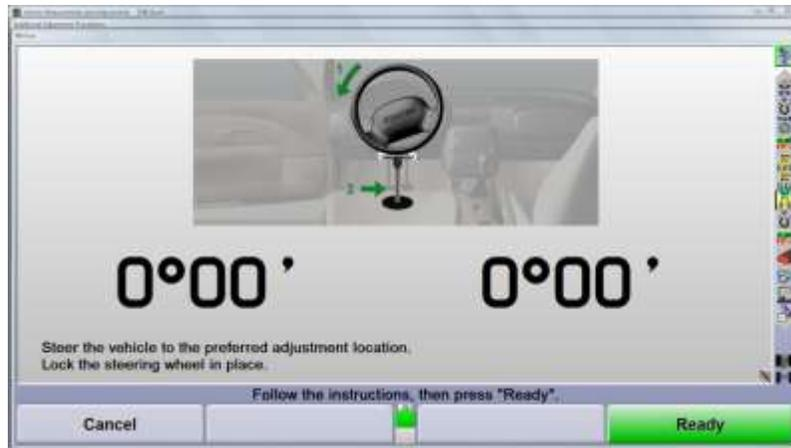
Follow the instructions on the display. Securely lock the front wheels in place after steering to the desired position. This may require using the ignition lock.
