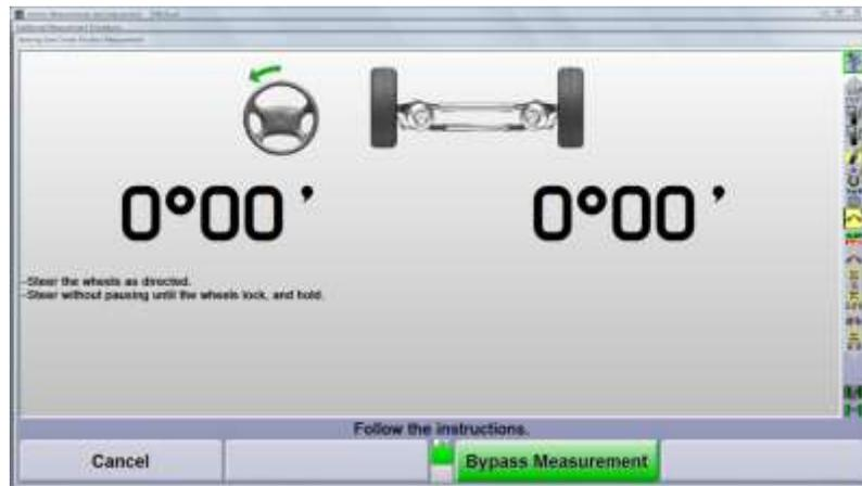
Steer the wheels as directed with a steady motion until maximum steer angle is achieved to the left. Hold the wheels until the display indicates to steer right.
