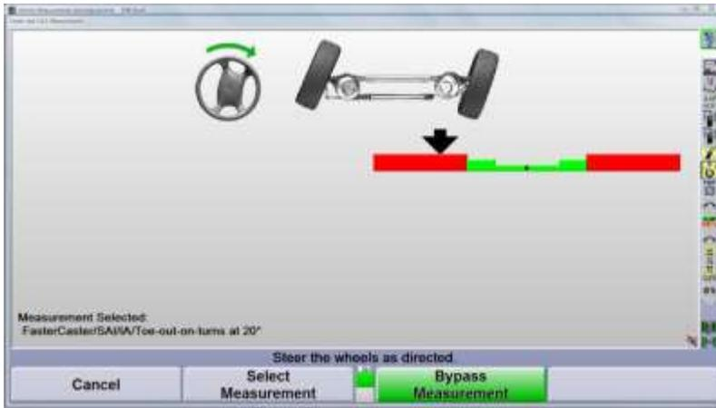
Steer to the right as directed until the arrow is in the lower valley of the graph. Hold the wheels still until the bar graph changes.
