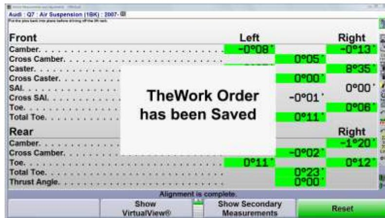
Conclude the alignment process by selecting the "Reset" softkey.
