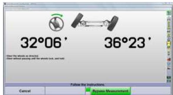
The final maximum steer measurement is made at this screen.
