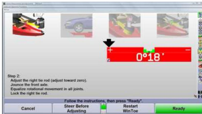
The toe adjustment display is shown with the same required change displayed before the front wheels were steered. Adjust toe and follow the instructions. Press K4 "Ready" when ready to adjust the left tie rod.
