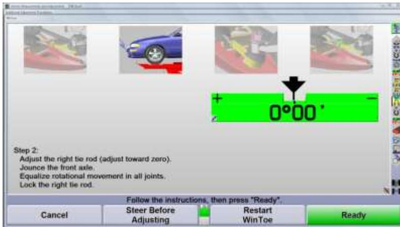
Steer the wheels to the position desired to access the left tie rod adjuster.
