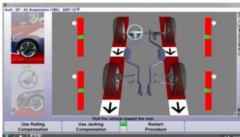
The lift rack should be level during the compensation process. The front turnplates and rear slip plates should be locked.
