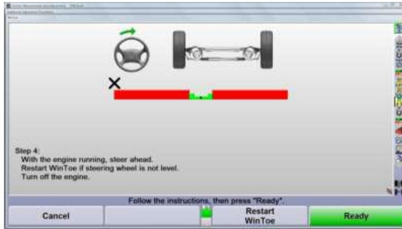
Verify the steering wheel is centered when the arrow is in the center of the bar graph.
