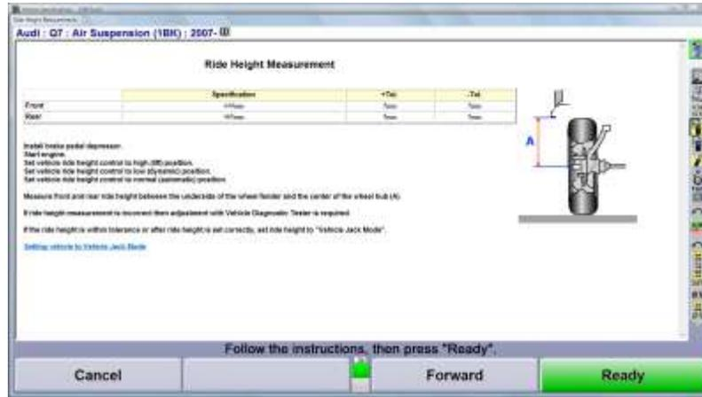
Current ride height values may be manually entered via the keyboard or electronically entered using Hunter's Live Ride Height targets..
