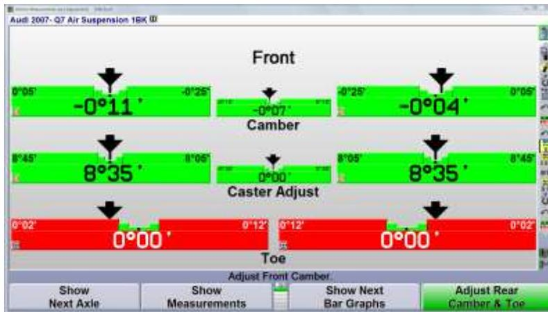
The "Raise Selected Axle" function may be used to make the adjustment easier. This is discussed in further detail later in this manual.
