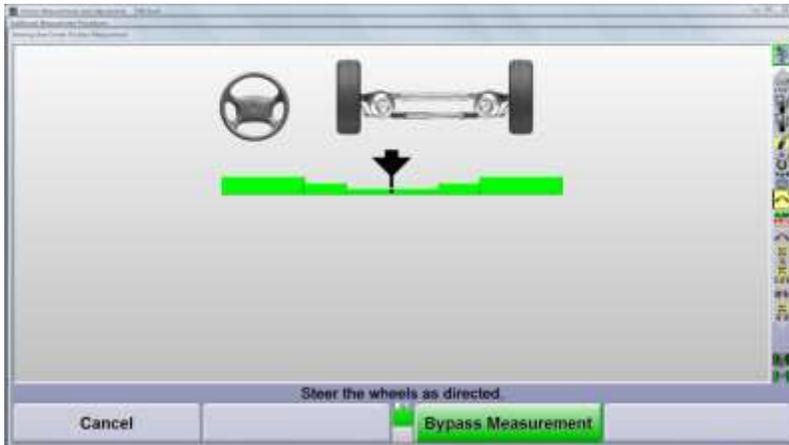
Steer back to the left until the arrow is centered in the bar graph. Hold steady until the screen changes.
