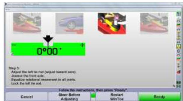
Be sure to jounce the vehicle and equalize the tie rod rotation after making an adjustment.
