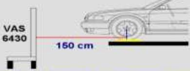
Assemble the VAS 6430 calibration fixture and set it approximately 150cm +/- 2.5cm ahead of the vehicles front axle centerline.
