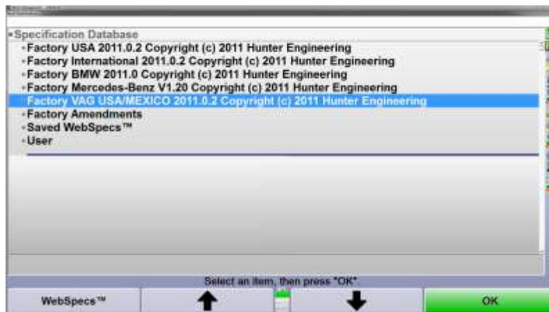
Use the K2 and K3 softkeys or the mouse to select the desired model from the Factory Specification database. It is crucial to select the exact vehicle with the exact options, such as wheel diameter, sport suspension, etc.
