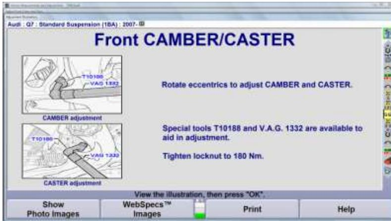
WinAlign will open the "Control Arm Monitor" program to make the adjustment easier. Follow the instructions on the display to adjust left and right camber/caster.
