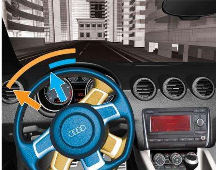
The central component is a superposition gear integrated into the steering column and driven by an electric motor. This harmonic drive gearing modifies the steering ratio in response to the car's speed. When you're parking, one turn of the wheel covers the full range of motion. At highway speeds, the same range takes four turns.
